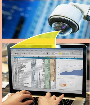
After implementing automation, live CCTV camera footage is continuously monitored in real time. The system automatically detects incoming and outgoing vehicles, identifies vehicle types, and extracts number plates using AI-based computer vision. Entry and exit time stamps are captured automatically, and the system matches the same vehicle during exit to calculate the total time spent inside the factory.
